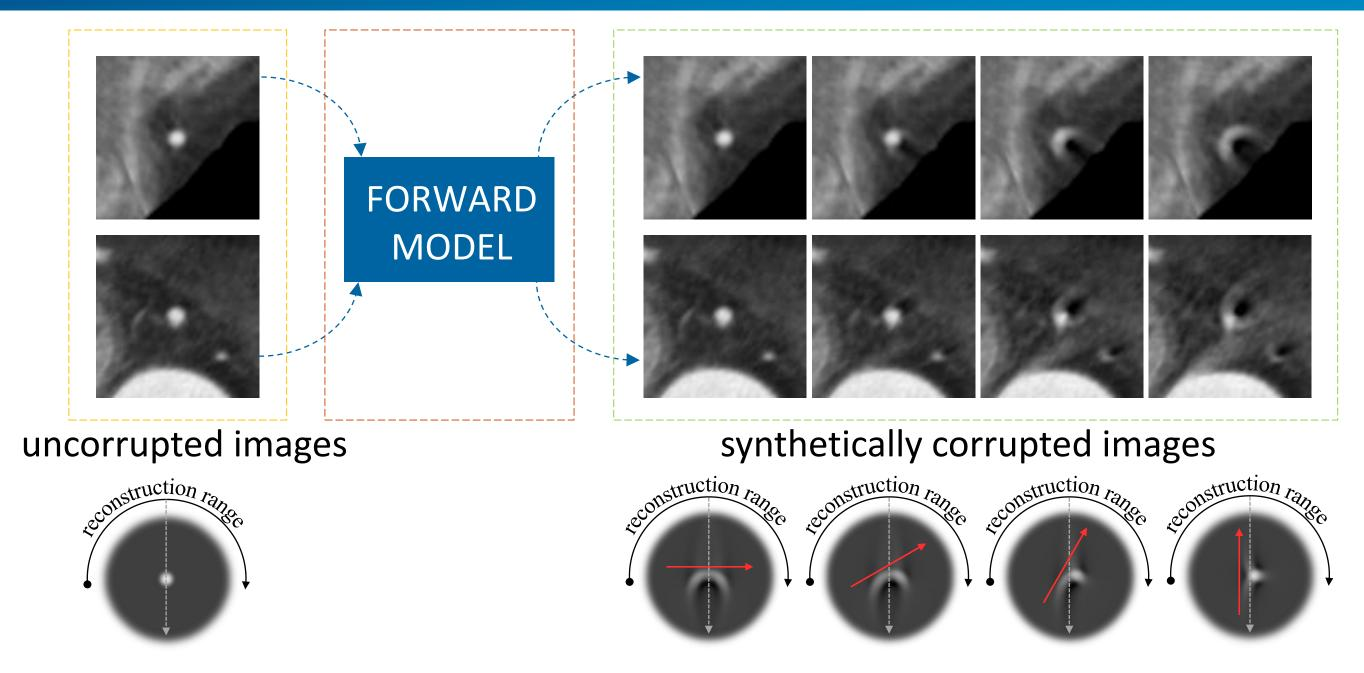
Main idea: Forward model [6, 7] introduces artificial motion to high quality CT cases to generate the required input and label data for supervised learning
