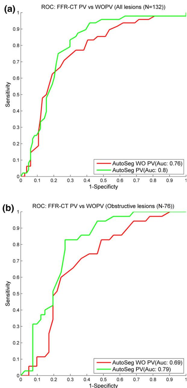
FIG. 7. ROC curves of cross-sectional area stenosis and flow simulation based on automatically generated 3D modes of the coronaries with and without accounting for the partial volume effects (PVE) using invasive FFR  $\leq 0.8$  as the reference for: (a) entire dataset, and (b) for lesions classified as obstructive (cross-sectional area (CSA) stenosis: 50–90%). [Colour figure can be viewed at [wileyonlinelibrary.com](http://wileyonlinelibrary.com)]
