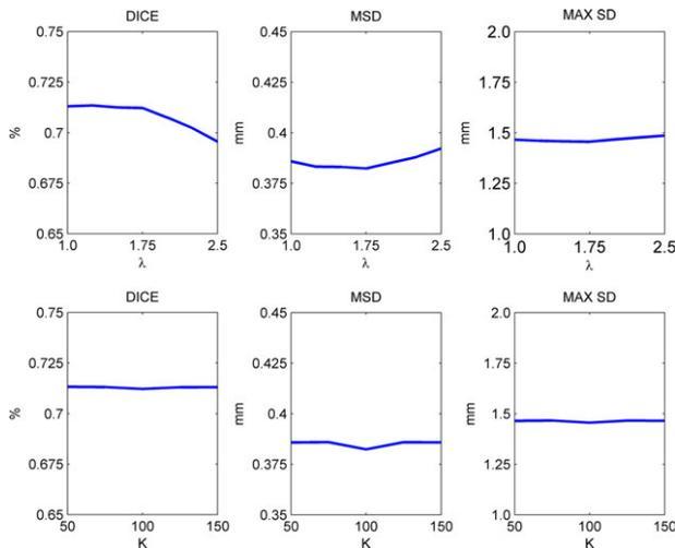
FIG. 4. Segmentation performance measures as a function of the two key parameters of the algorithm:  $\lambda$  [Eq. (5), upper row] and  $K$  [Eq. (6), bottom row], over the 18 training cases from the MICCAI 2012 dataset.<sup>12</sup> Measures used are the Dice coefficient (left column), the mean surface distance (mid column), and the maximal surface distance (right column). [Colour figure can be viewed at [wileyonlinelibrary.com](http://wileyonlinelibrary.com)]
